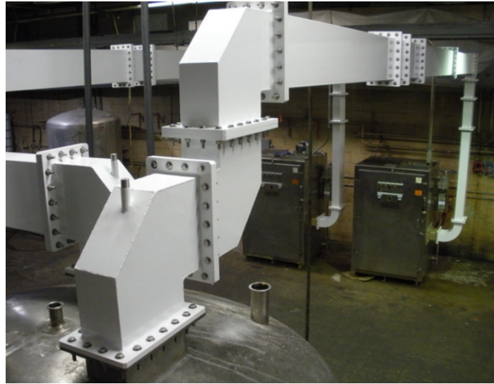
Figure 1: Waveguides deliver microwaves at 915 MHz frequency to top of a vertical vessel for processing products
