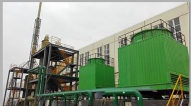
Figure 3: C1-containing gas absorption for producing HCl and NaClO 2 solutions
