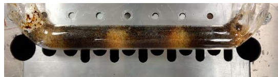
Figure 4. Charred and not charred regions in pine sawdust sample after microwave treatment.
