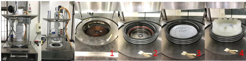
Figure 1. The MAPIH simulator, and assembly of processing cavity.
