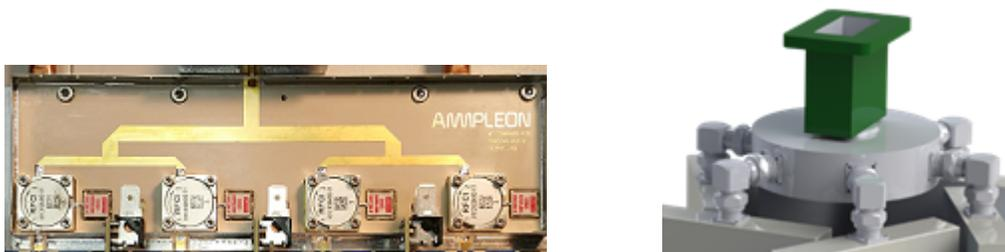
Figure 1. Internal four way microstrip combiner for 60dBm[1] (a) and radial combiner combining 60dBm systems for multi kilowatt output[1] (b).
