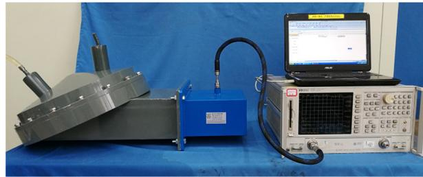
(a) water load under testing
