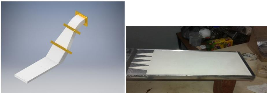
Figure 1: Evanescent field applicator, based on an alumina dielectric resonator, seated into the applicator housing and fed from a standard WR340 wave guide (left) an overview of the applicator design and (right) a photograph of the alumina block inside the applicator housing.
