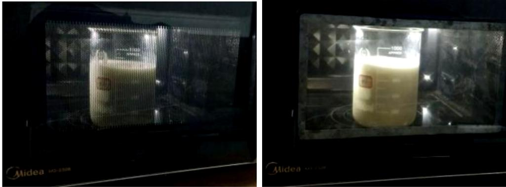
Figure 2. Photographs of milk being heated in a microwave oven with (a) the normal metal grid and (b) the transparent conductive film observation windows.
