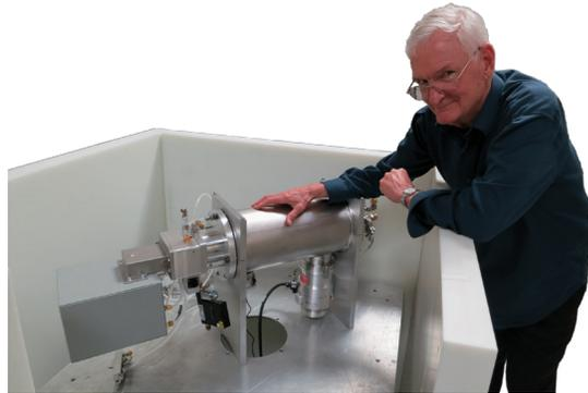
Figure 1. A DD neutron generator. From left to right: magnetron box, waveguide+matching stub, ECR ion source, acceleration chamber. White material surrounding generator: neutron shielding.
