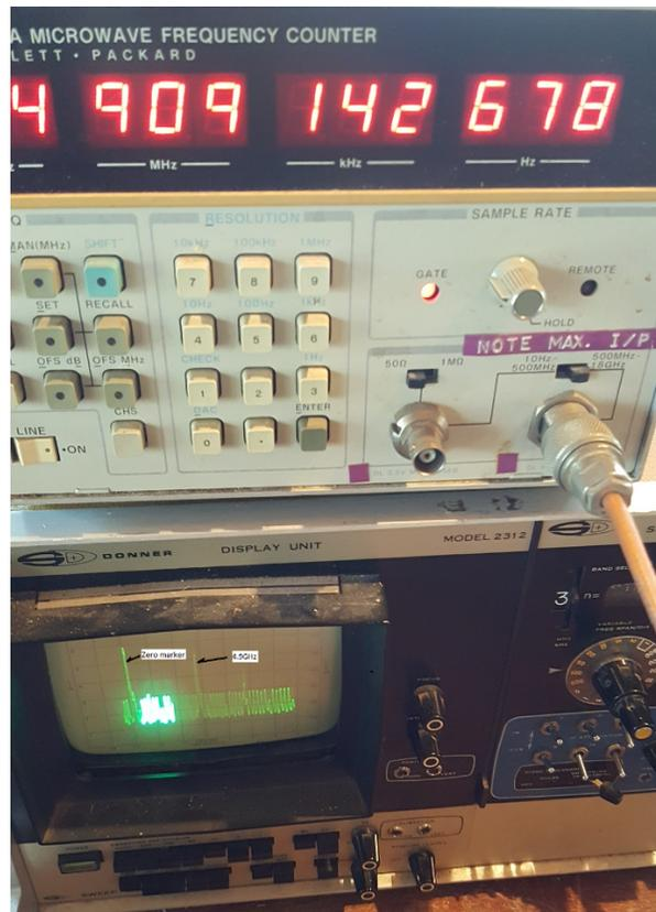
Figure 1. The converted frequency is shown by a frequency counter and a spectrum analyzer.
