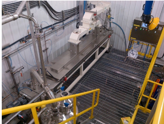
Figure 1: Continuous-Flow Industrial-Scale MAP™ Extractor
