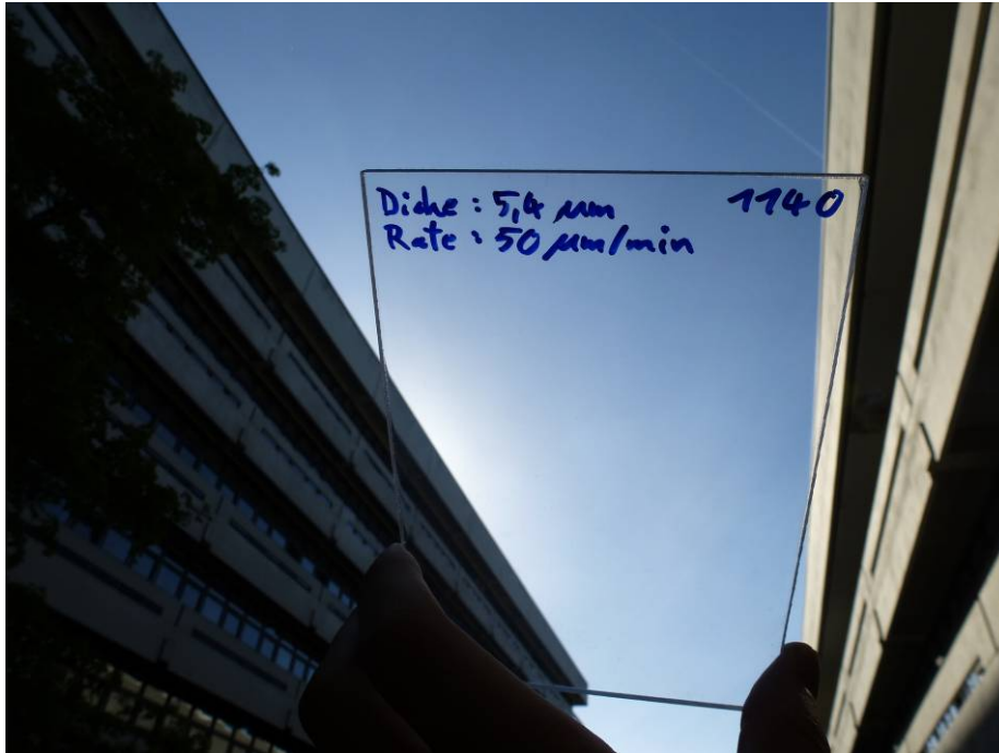
Figure 2. Polycarbonate plate with additional quartz-like protection layer deposited in a low-pressure microwave plasma process showing almost 100% transparency.
