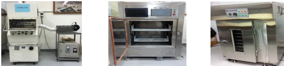
Figure 1. (a) RF hot air heating equipment, (b) Microwave drying oven, (c) Cold air drying oven.
