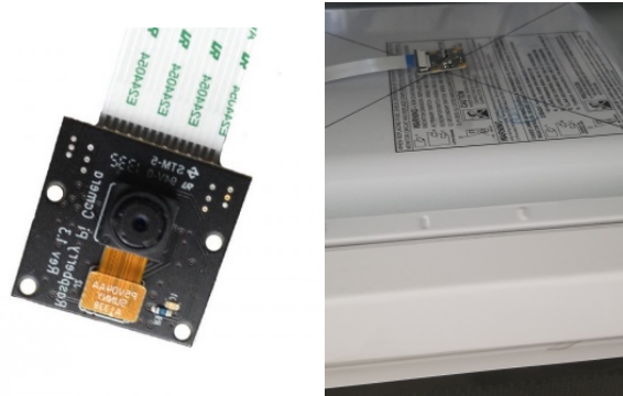
Figure3. a).The Raspberry PI NoIR Camera, at under $30 provides a lower cost alternative to a FLIR and is noted by its black silkscreen, and b). The camera in-situ atop the oven cavity during testing.
