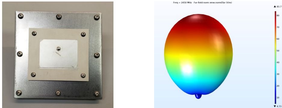
Figure 1. (a) Circularly polarized high power patch antenna, and (b) far field plot of same antenna
