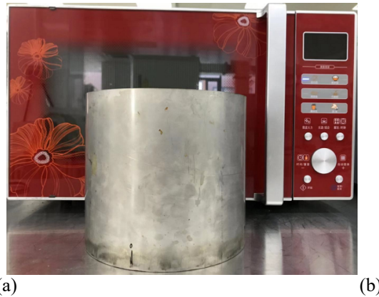
Figure 1. Microwave oven and the cylindrical cavity.
