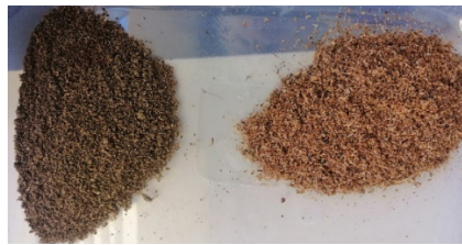
Figure 3 Appearance of milled product after conventional treatment (left) vs RF treatment (right)
