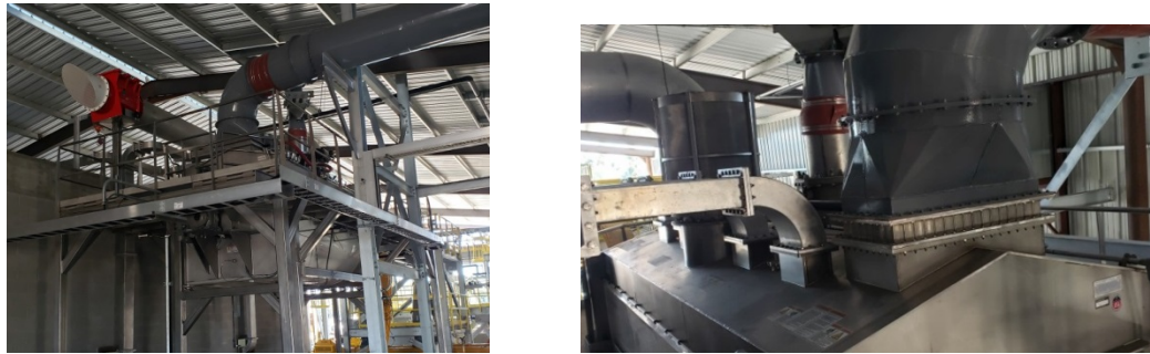
Figure 1. a) The 400 ft 3 applicator. b) View of the top side of the applicator. Top connections include four waveguide feeds, material fill port, and exhaust ports.
