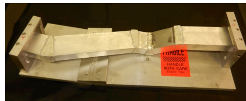
Figure 4. Waveguide fixture used for pre-braze tack-up and post-braze machining.
