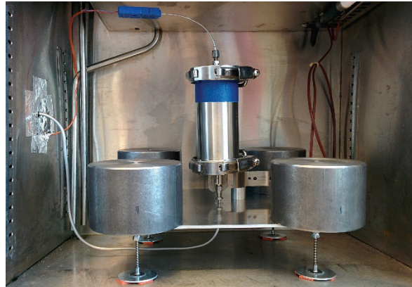
Figure 2. Initial design of the vibration-isolated test cell.
