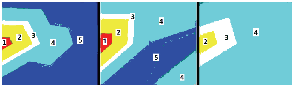
Figure 5. Thermograms of cavity B. 6 cm height (left), 10.5 cm (center), and 11 cm (right). Temperatures: 1) 175-200°C, 2) 150-175°C, 3) 125-150°C, 4) 100-125°C, 5) <100°C.
