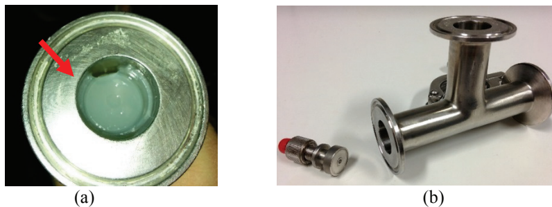
Figure 1. The formation of air bubble in a horizontally oriented test cell: (a) air bubble formed near the coaxial probe during solidification of agar gel and (b) the horizontal setup.
