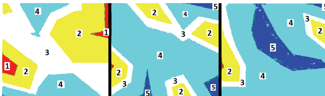
Figure 3. Thermograms of cavity A. 6.5 cm height (left), 13 cm (center), and 16.5 cm (right). Temperatures: 1) 110-120°C, 2) 90-110°C, 3) 70-90°C, 4) 50-70°C, 5) <40°C.
