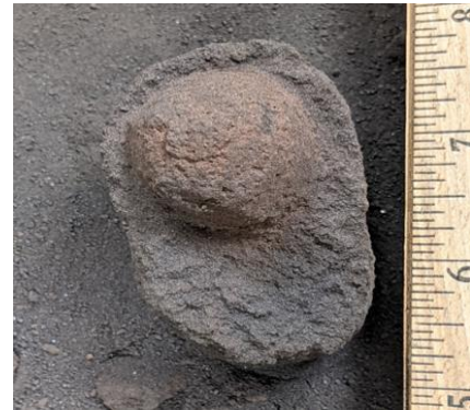
Figure 4: Sintered JSC1-A simulant. Upper surface was approximately 3/8" below the surface.
