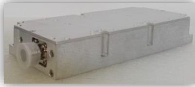
Figure 1. Photo of the 2,450MHz module, elementary item for scalable architectures.
