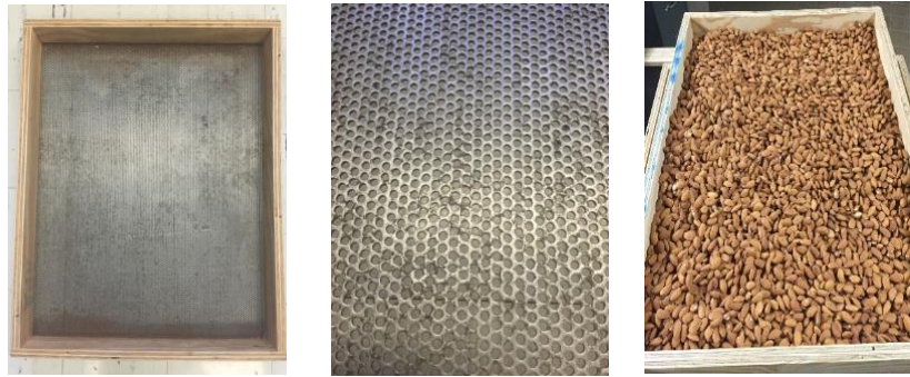
Figure 1. Tray with perforated bottom to allow almond kernels to absorb humidity from surrounding air.
