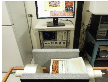
Figure 3. Free-space measurement arrangement.
