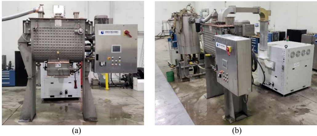
Figure 1. Views of the overall test setup (a) and the horizontal mixer (b).
