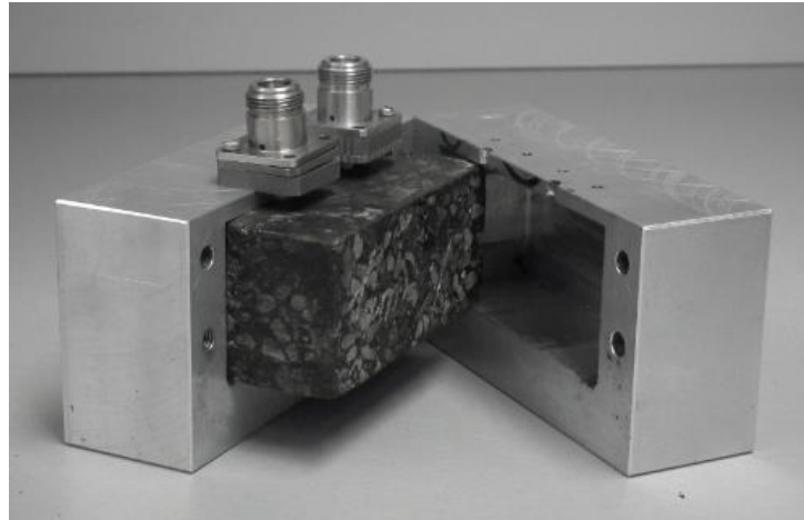
Figure 4. Rectangular resonator with an asphalt sample completely filling the cavity (after [2]).
