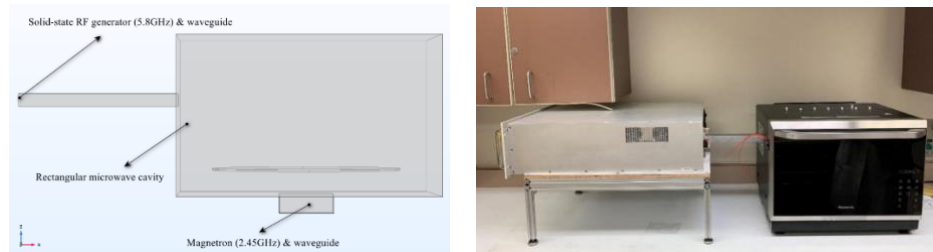
Figure 1. A dual-frequency domestic microwave oven
