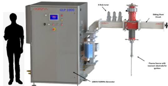
Figure 1. View of the 915 MHz 100 kW microwave plasma torch.
