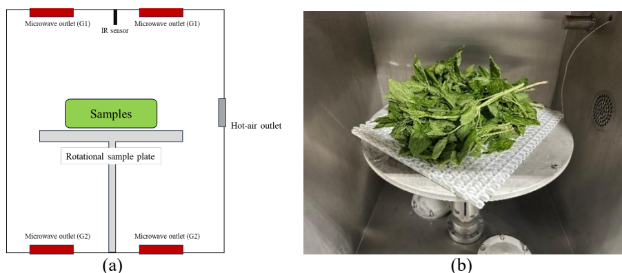
Figure 1. Schematics of the chamber in FL12000 (a) and basil in FL12000 (b).
